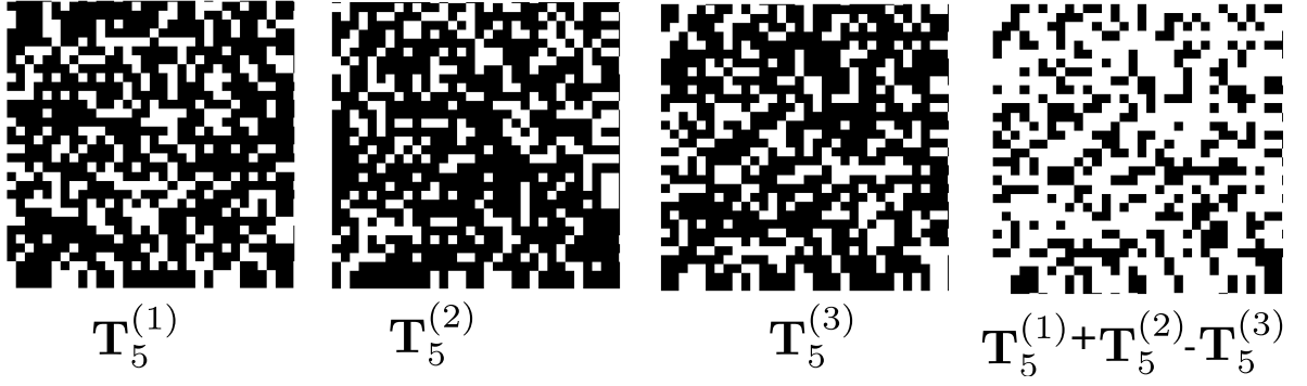
Figure 6.7: A 64 \times 64 window of the designed coded aperture with the new design approach is depicted for the source number 5 when K = 3 shots are considered.
